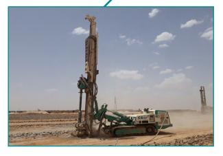
KOMATSU PC210-8 equipped with powerful drilling mast & T20EP rotation head (Max. Torque 15.2 KN.m)
